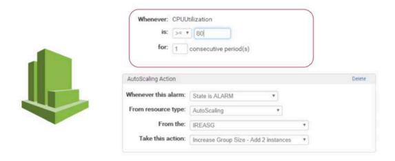
Also set a rule when CPU utilization goes below 20% for more than 5 minutes for example. We can also specify the rule as a utilization target, and apply boundaries in terms of maximum and minimum instances.
