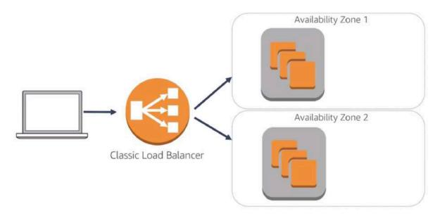
The elastic load balancer provides a single point of access to the backend instances. Need to set up an alias record to point our domain CName to the endpoint for the elastic load balancer.
