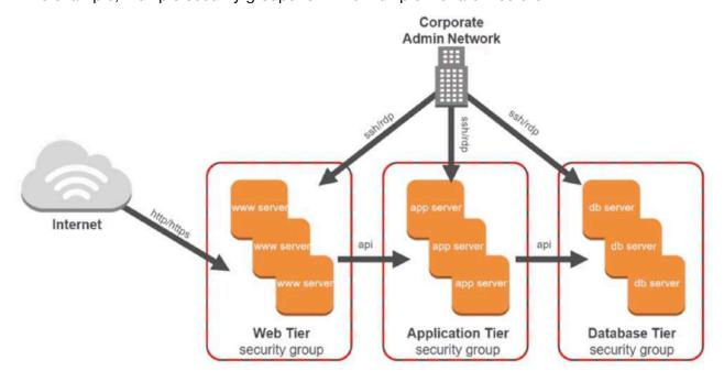
Typically here, traffic is allowed from the internet. The application Tier only allows connexion from the web tier, and the database tier only accepts traffic form the application tier. An administration rule has been created to allow connexion using SSH ports from the corporate network.
