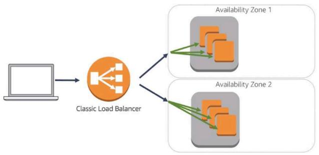
Internal load balancer: has a DNS name that resolves only to private nodes so it can only be
